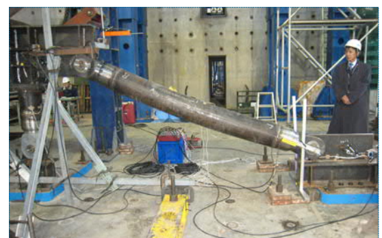
\phi 244.5 \times 8 L=2530 (slenderness ratio 30)
