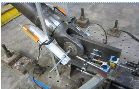
\phi 244.5 \times 8 L=2530 (slenderness ratio 30)
