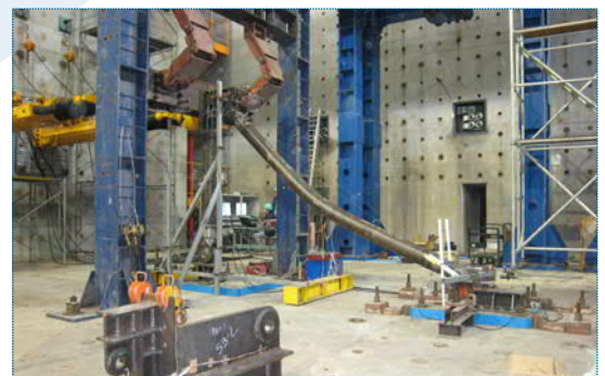
\phi 244.5 \times 8 L=4852 (slenderness ratio 58)
