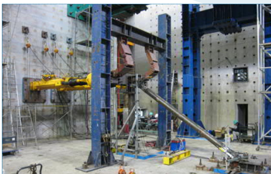
\phi 244.5 \times 8 L=4852 (slenderness ratio 58)
