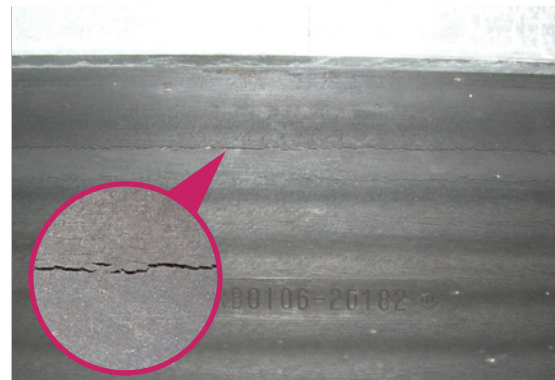
rubber bearing with ozone cracks
