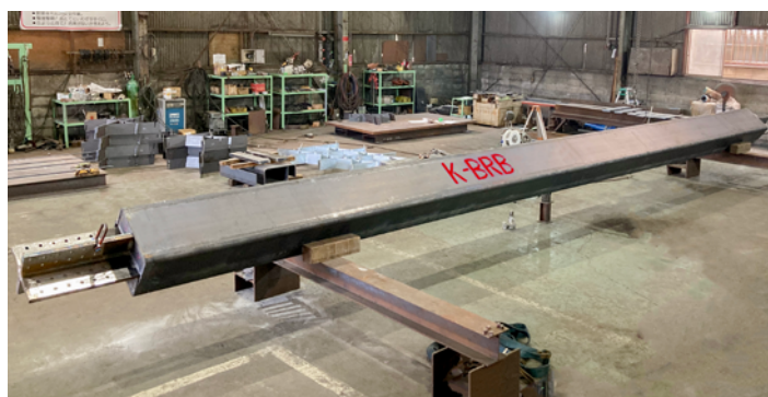
K-BRB manufacturing (Length 12m)
