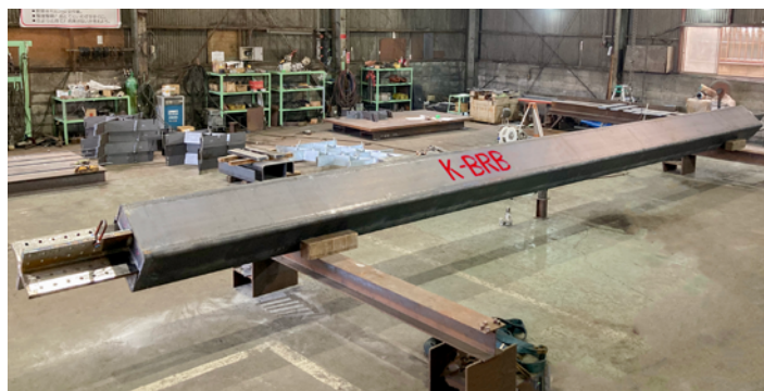
K-BRB manufacturing (Length 12m)
