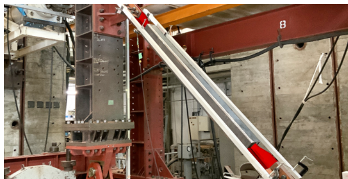
K-BRB performance test at Kanagawa University(Japan)
